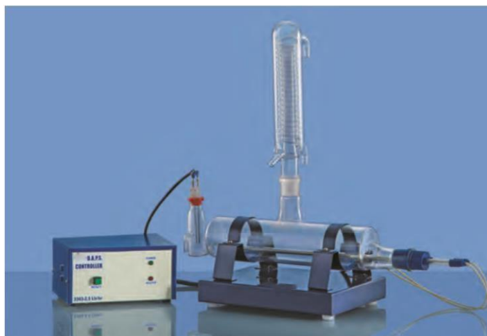
2001. A1.01 - All Glass Single Distillation Units, with Borosilicate Boiler, Borosilicate Condenser & Quartz Heater, Horizontal Type.
