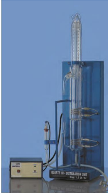
2001. A4.01- All Quartz Double Distillation Unit, Demountable Boiler Panel series, Vertical Model,
